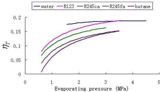
**Fig.6 Total Heat Recovery Efficiency with Respect to Evaporating Pressure ( $T_{in}=450^{\circ}C$ )**
