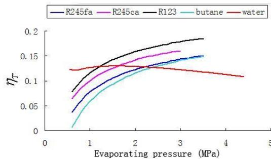
**Fig.8 Total Heat Recovery Efficiency with Respect to Evaporating Pressure ( $T_{in}=350^{\circ}C$ )**
