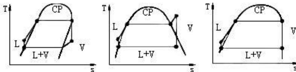
Fig.5 T-S Diagram Dry, Wet and Isentropic Fluid
