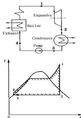
Fig.2 Structure of Rankine Cycle System and its Ideal T-S Diagram
