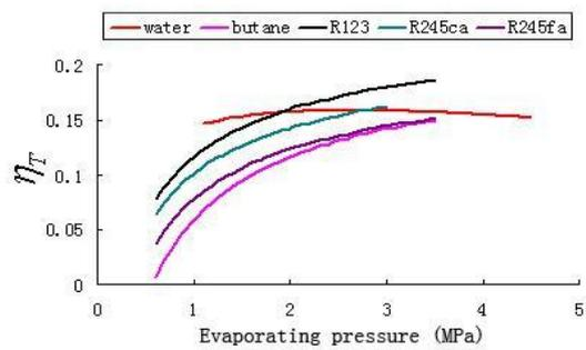
**Fig.7 Total Heat Recovery Efficiency with Respect to Evaporating Pressure ( $T_{in}=400^{\circ}C$ )**
