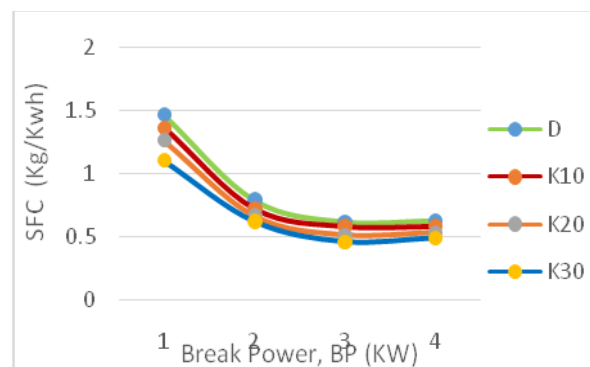
Fig 4- Plot of Specific Fuel Consumption, SFC vs Break Power, BP
