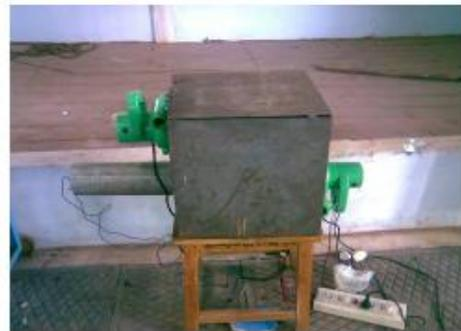
Figure 2. Solid Desiccant Dehumidifier Set Up
